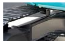
●Special crawler frame designed is easily cleaned of mud.
