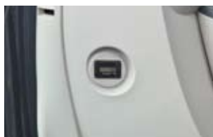
Hour meter can be checked while standing on the ground
