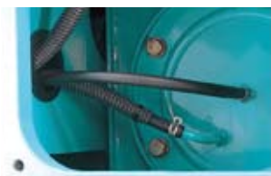
Fuel tank equipped with bottom flange and large drain valve
