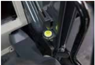
●Level indicator that shows degree of machine tilt
