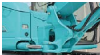
Swing bracket ●Large, thick cast-iron swing bracket
