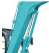
Boom: ●Guard plate for boom cylinder
