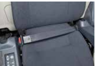
●Retractable seatbelt requires no manual adjustment
