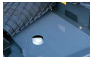
Washer fluid tank located under the cab floor mat.
